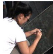
Clear plastic tape is used to collect a sample. The sample is analyzed with a microscope to determine whether the substance is mold or soot. (photo courtesy of Terry Brennan)
